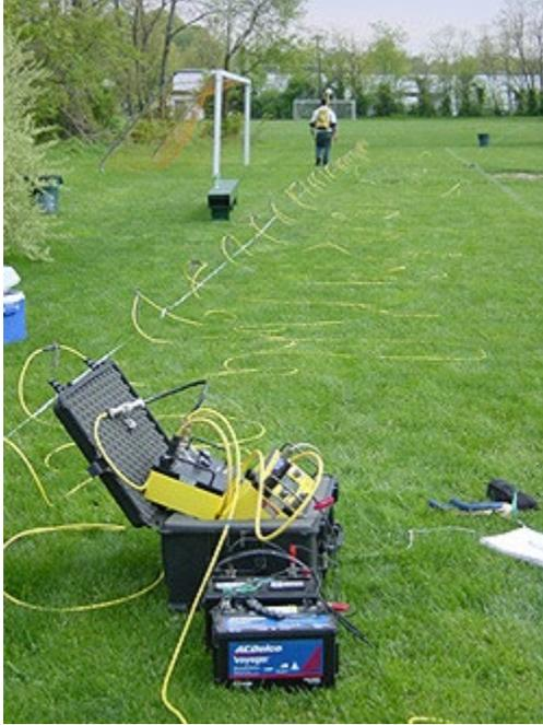
Figure 4. DC Resistivity data acquisition system deployed for site characterization (<http://water.usgs.gov/ogw/bgas/toxics/NAWC-surface.html>). *This image is provided for demonstration purposes, and is not intended as an endorsement for use of this product.*
